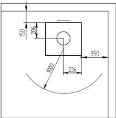
Distance to combustible WITH insulated flue
